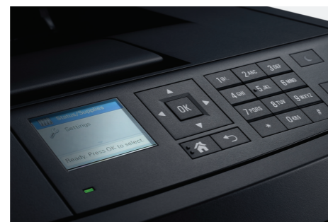
Ease of operation with intuitive 2.4 inch (6.09 cm) LCD with numeric pad.
