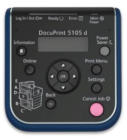
The simplified control panel of the DocuPrint 5105 d makes on-printer operations quick and easy.
