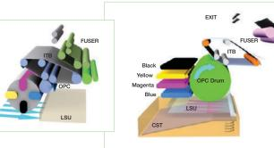
NO-NOIS® Technology Thanks to Samsung's revolutionary Non Orbiting Noiseless Optical Imaging (NO-NOIS<sup>®</sup>) System, the new CLP-So0 series printers are free from loud mechanical noise. The toner is stored in fixed cartridges that transfer colour on to the Image Transfer Band (TB) in one simple step, via a smoothly rotating OPC drum. A technical innovation that soothes both ears and nerves.
